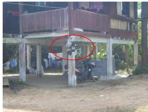
BreadCrumb® attached to existing structure in the refugee camp also located in the city of Khao Lok. This BreadCrumb® meshed to one other BreadCrumb® in the administrative building located 300 meters away. This network also provided internet access via satellite uplink for the refugee camp.
