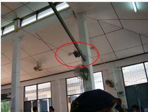
BreadCrumb® located at Young Yao Temple identification and reclamation center in the city of Khao Lok. There were a total of three BreadCrumb® used to establish the network which was connected to the internet via a satellite uplink.
